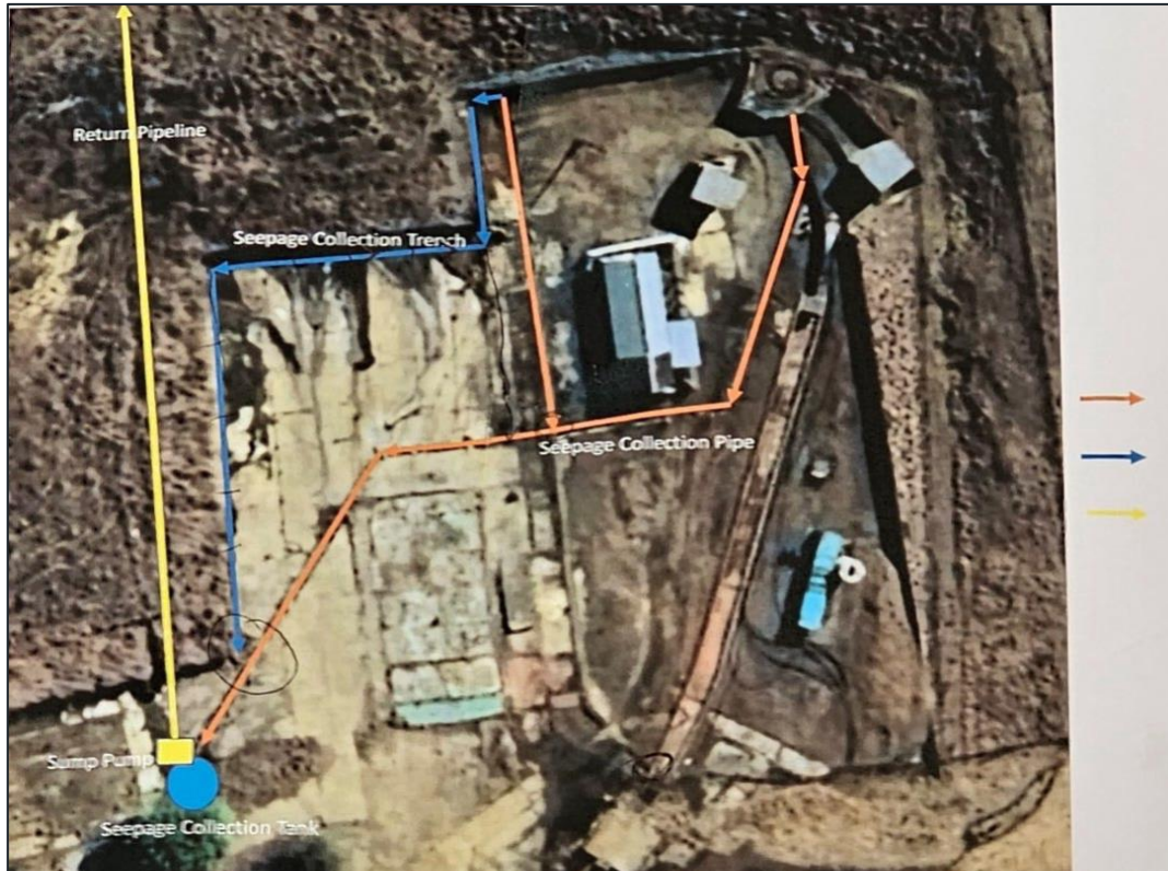
Figure 2-5 – Seepage collection and sump at the main adit, April 2023
