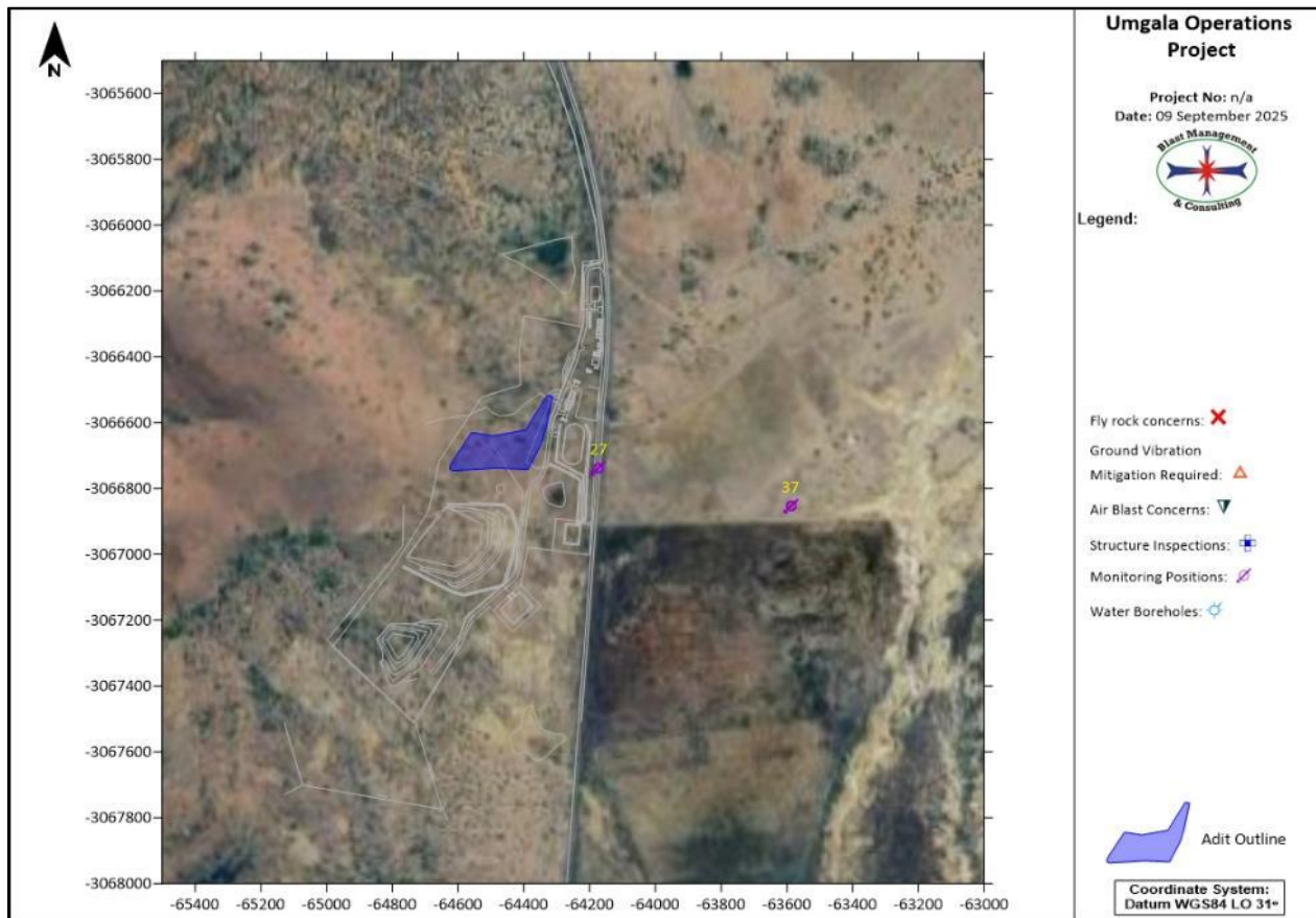
Figure 97: Suggested monitoring positions – Adit area
